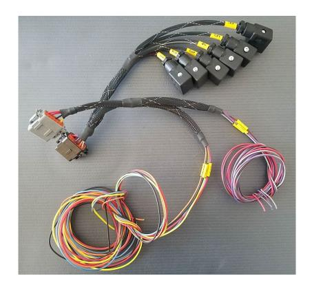
A manual reverse version will look similar, only missing the cap that is labeled "R" and a single wire that is for the pneumatic reverse button described later.
