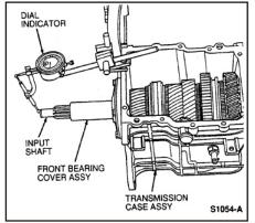
2. Remove four front bearing retainer bolts.
