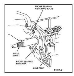
3. Remove front bearing retainer.
